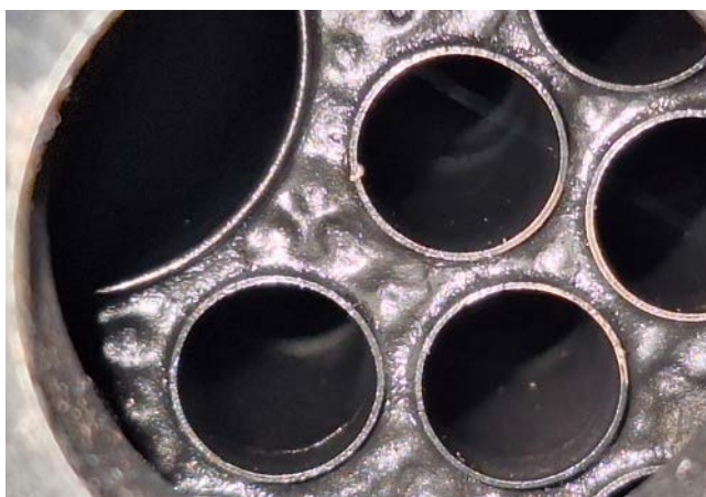
Bubble and crack formation (left) and significant discolourations (right) – typical damage symptoms of thermal overstressing
