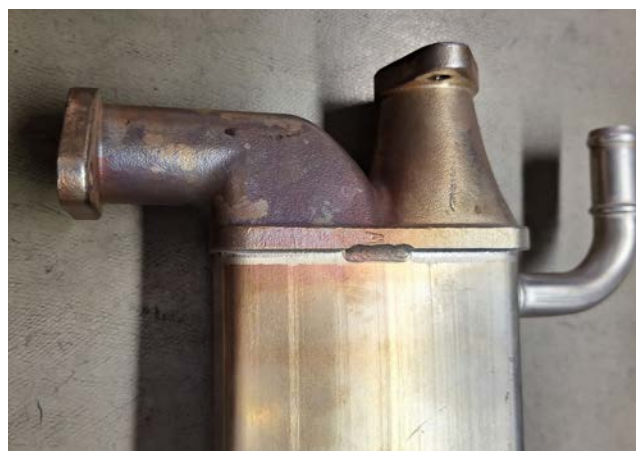
Bubble and crack formation (left) and significant discolourations (right) – typical damage symptoms of thermal overstressing
